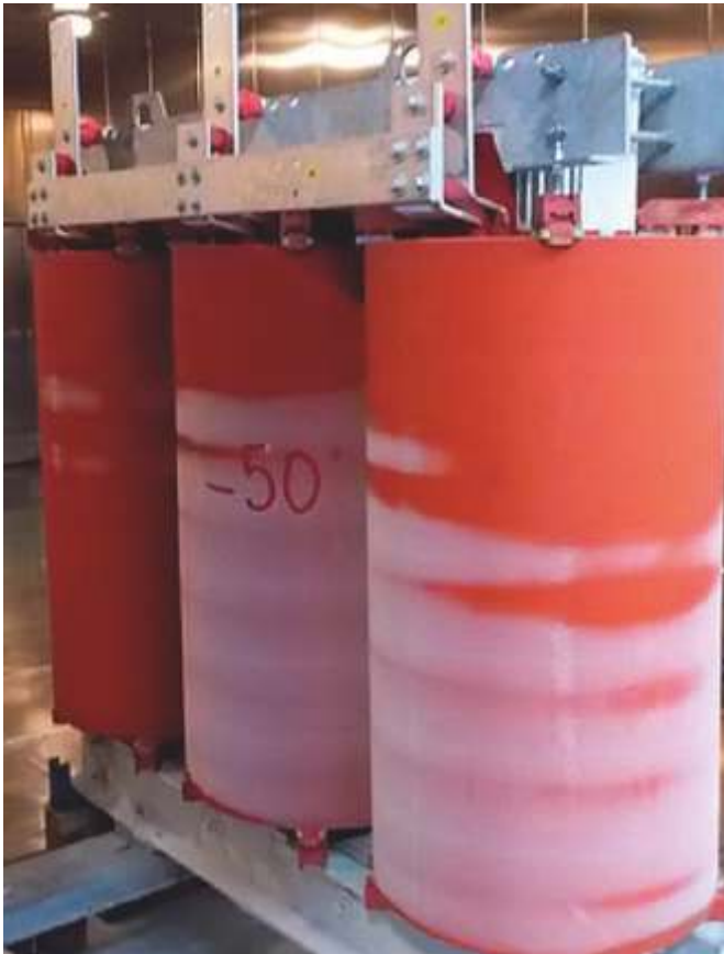
Tesar transformer during climate test
